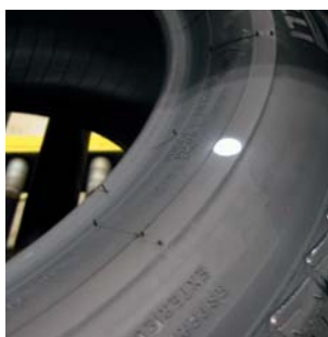
High-point marking on automobile tires
