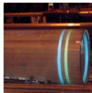
Colored ring marking on steel pipes
